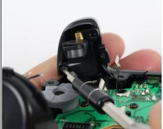
• Unscrew the two 7mm T6 Hex screws located on underside the triggers.
