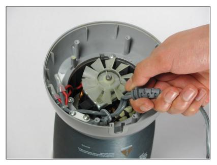
• Lift the power cord to remove it from the side slot on the curved base.
