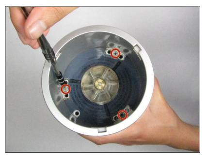
Remove the three 15mm screws with the Philips Head 2 Screwdriver.
