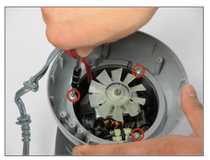
Use a #2 Phillips Head Screwdriver to remove the three 10mm screws that keep the base in place.
