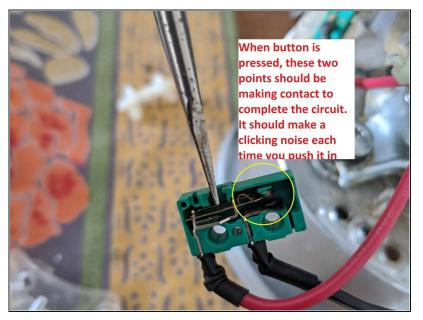
Open up the green switch. The metal tab and black button will fall out. Fiddle around with the metal switch on the inside to snap it back into place and then reassemble carefully. It should make a clicking noise.
