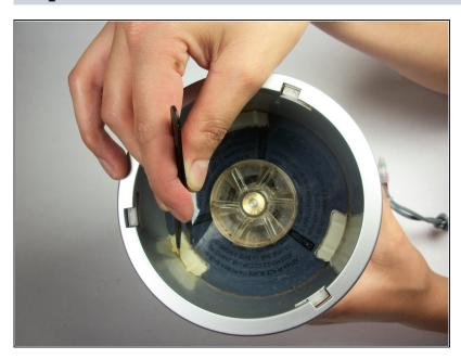
Place the NutriBullet powerbase on the table so that the three rubber screw covers are visible along the bottom of the well. Remove the covers using either tweezers or your fingers.
