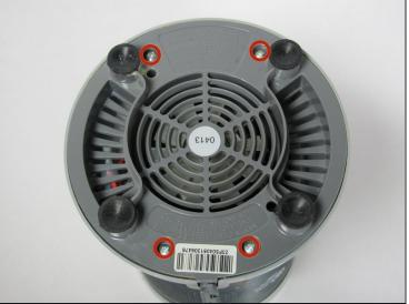
• Use a #2 Phillips Head Screwdriver to unscrew the four 10 mm screws located on the bottom of the power base.
