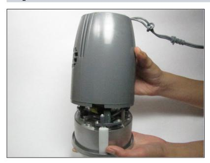
Turn the NutriBullet powerbase upside down and remove the plastic casing by lifting it up. You may have to wiggle the casing in order to break away any hardened material.
