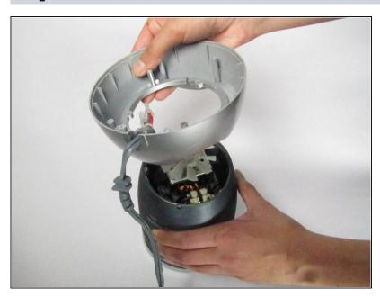
Use slight tension to remove the curved base by lifting it upward off of the outside casing.
