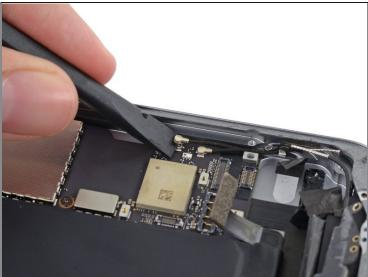
Use the flat end of the spudger to pry the antenna connector up from its socket on the logic board.
