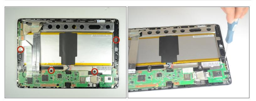
• Remove the four 2 mm Phillips #00 screws holding the battery tray in place.
