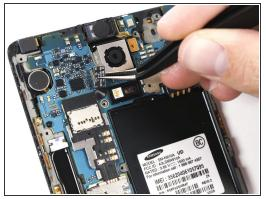
• Use a set of tweezers or the flat end of a spudger to disconnect the two ribbon cable connectors.
