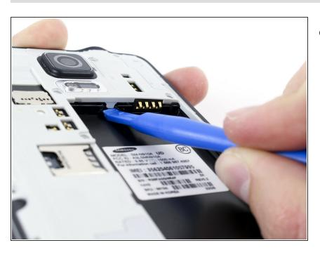
Use a plastic opening tool to loosen the clasps around the battery housing.
