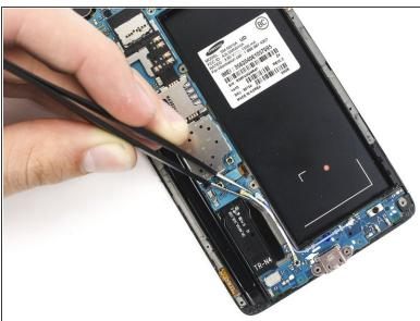
Use a set of tweezers to remove the two antenna cables.
