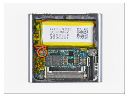
Remove the single 1.9 mm Phillips screw securing the logic board to the outer case.
