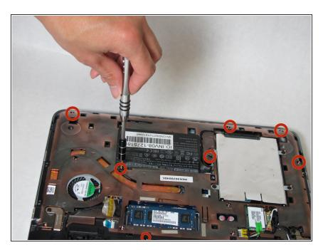
Unscrew all screws attaching the fan to the metal backboard.
