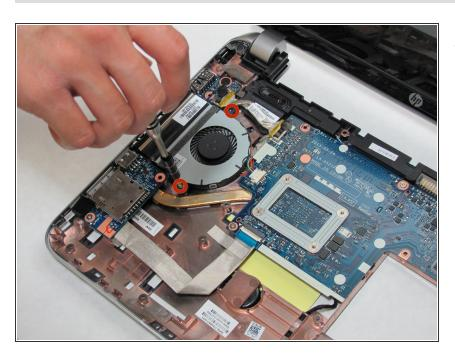
Unscrew the two screws that keep the fan in place.
