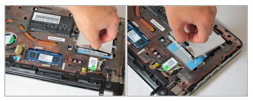
• Carefully lift the hard drive up by holding the tag shown here.
