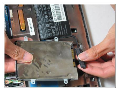
Remove the final attachment to the hard drive located at the end shown here.
