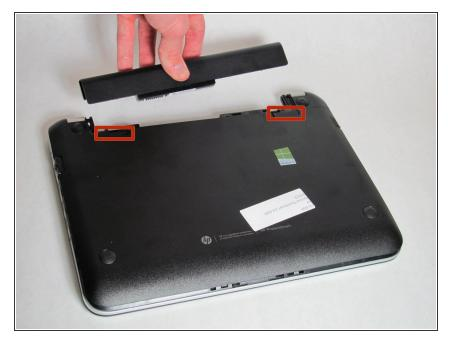
Remove battery by pushing the two tabs and pulling the battery outwards slowly but firmly.
