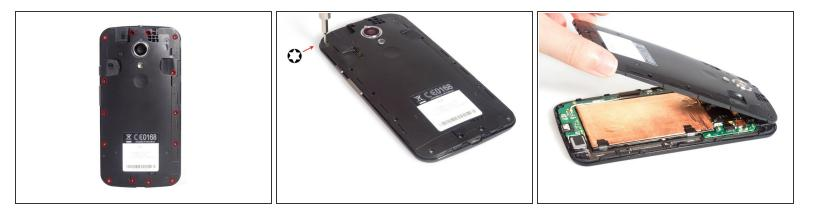
• Twist off all 14 screws together and remove the back frame easily. But the screws feature different lengths, you'd better remember their positions.
