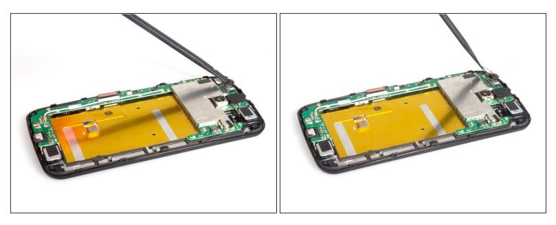
• Release sensor flex connector and front camera connector respectively.
