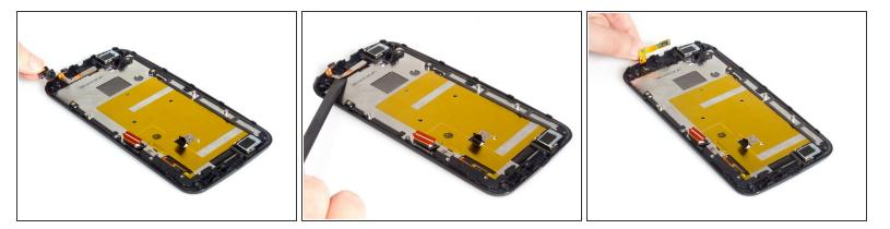
• Remove front camera and sensor cable.
