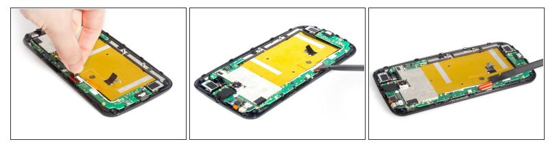
• Release LCD screen connector from motherboard.
