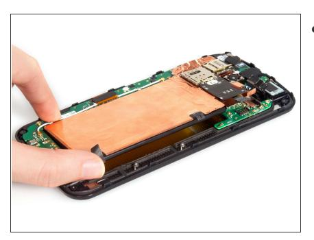
At that time, remove the battery with SIM & SD card reader assembly together.
