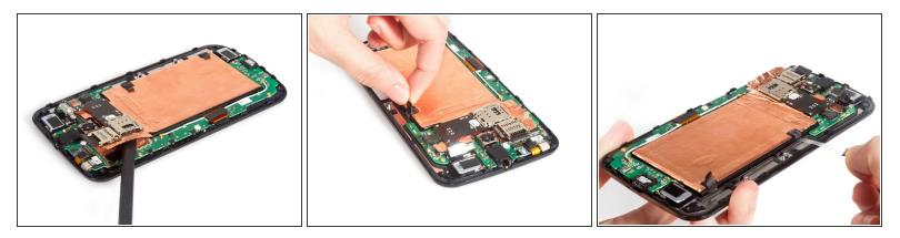
Loosen the platinum foil under SIM & SD card reader from plate. And then drag the stickers out which fix the battery.
