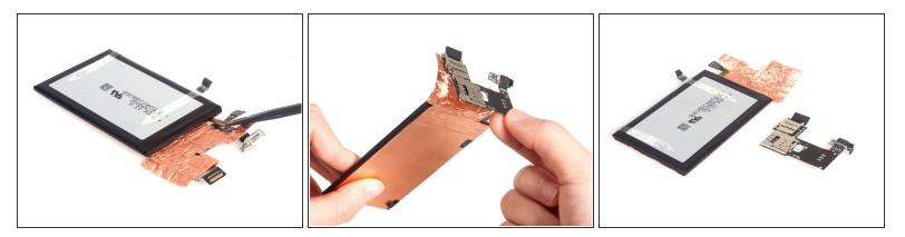
• Separate battery and SIM & SD card reader assembly.
