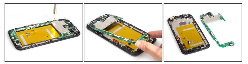
• Remove screws on the motherboard and the motherboard can be removed easily.
