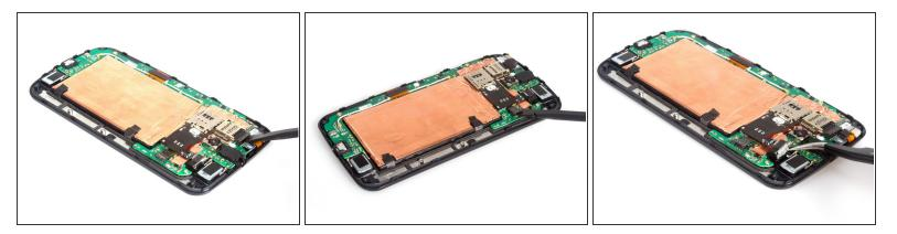
Release SIM&SD card reader connector and battery connector. And get the vibrator motor free from adhesive.
