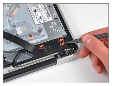
Use the tip of a spudger to pry the three antenna connectors up off the AirPort/Bluetooth board.
