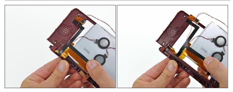
Holding the upper LCD and the cameras together, pull the cables through the hinge in the front bezel.
