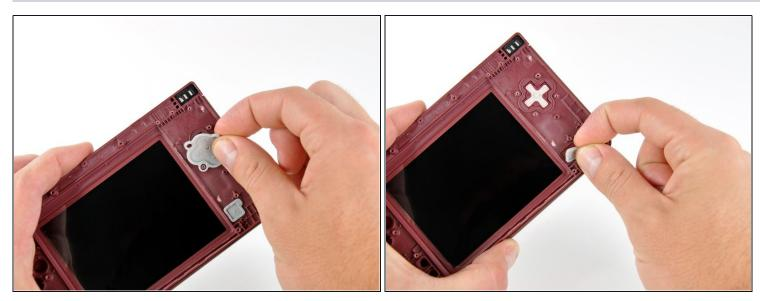
• Peel the rubber button pads off the backside of the D-pad and power button.
