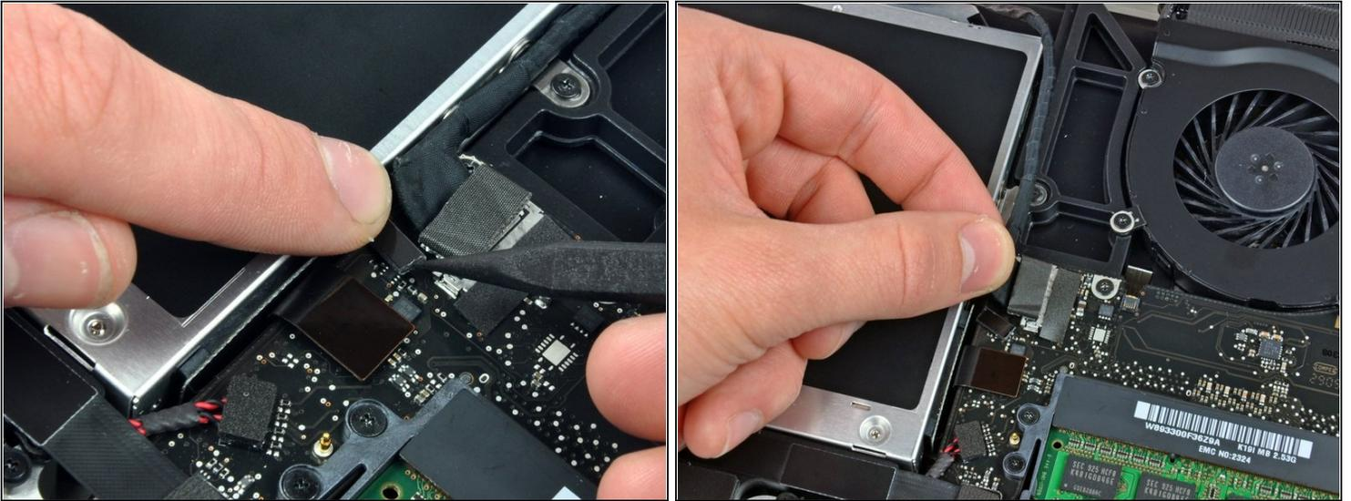
**⚠** Apple sticks a small strip of clear plastic with adhesive applied to one side to the logic board behind the camera cable connector to keep it in its socket. When moving it out of the way, be sure not to break any surface-mount components off the logic board.
