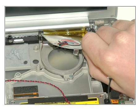
Lift the right fan out of the computer (the yellow tape will peel up with the fan).
