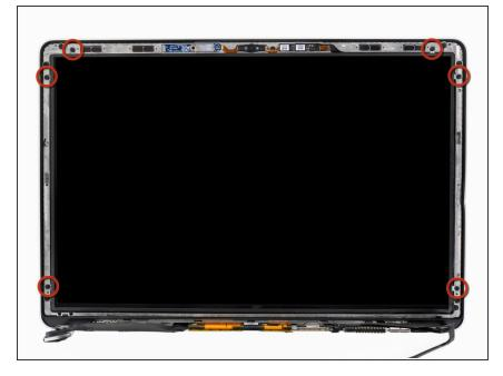
Remove the six 2.9 mm Phillips screws securing the LCD panel to the front bezel.
