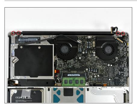
Remove the two outer 6 mm Torx screws securing each side of the display to the upper case (four screws total).
