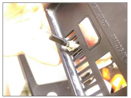
Insert the switch. In this example, a slot was removed from the vent to allow a larger switch. Make sure your switch is firmly attached and that its position will allow it to fit into the system.
