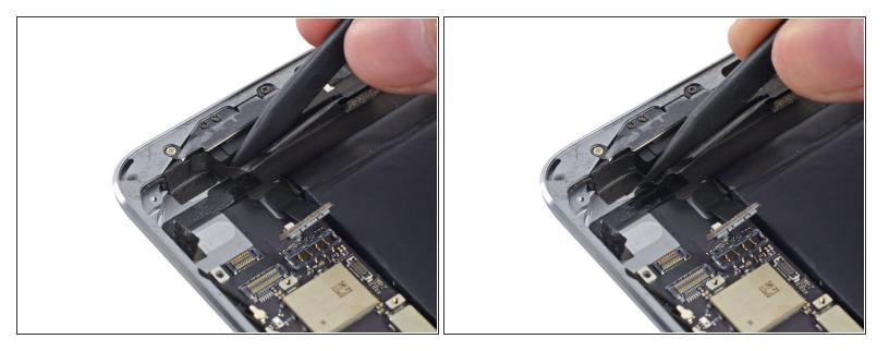
• Use the point of a spudger to separate the adhesive holding the antennas to the right speaker.
