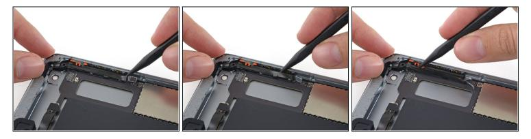
• Use the point of a spudger to separate the case button cable from the button cable mounting rail.
