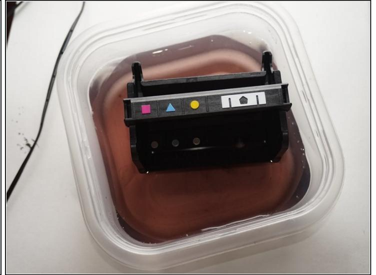
**⚠ Only use alcohol as a final option. It may damage the printhead seals! IF USED, FLUSH WITH CLEAN WATER 3 TIMES.**
