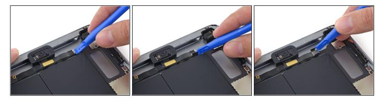
Use a plastic opening tool to fold the front-facing camera cable clips outward, away from the cable, freeing the cable connector.
