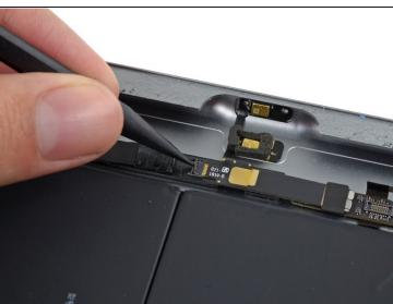
• Use the tip of a spudger to flip the microphone cable ZIF connector tab.
