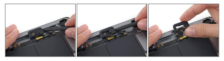
• Use the tip of a spudger to pry the front-facing camera housing up and lift it out of the case.
