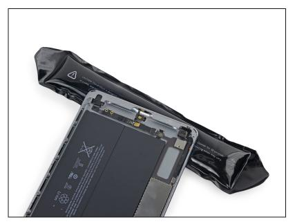
Heat an iOpener and lay the iPad on it, to heat the microphone adhesive.
