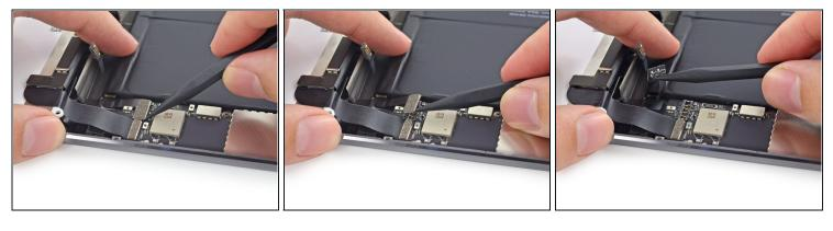
• Use the tip of a spudger to gently lift the battery connector up off its socket on the logic board.
