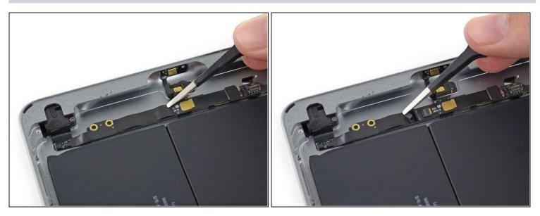
Use a set of tweezers to peel back any tape covering the dual microphone cable connector.
