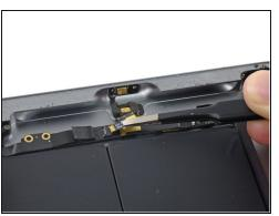
Slide one end of a set of tweezers under the microphone cable and pull it out of its socket.
