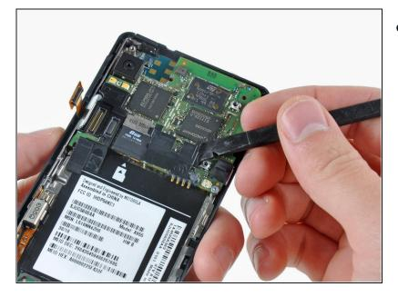
• Use the flat end of a spudger to remove the small black plastic piece stuck to the battery connector.
