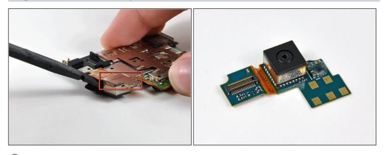
(i) Orient the motherboard so that the camera lens is face down.
