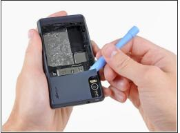
Every screw holding the Droid 2 together is cleverly hidden behind the many covers stuck to the rear of the device.
