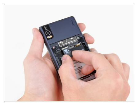
The Droid 2 comes pre-installed with an 8GB microSD memory card that can be easily slid out of its socket.
