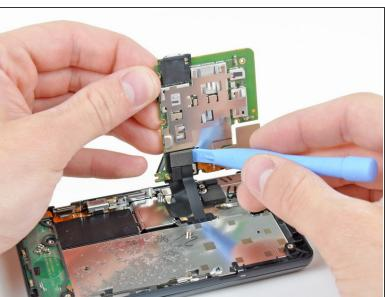
After removing the screws securing the motherboard to the phone and disconnecting the keypad ribbon cable on the opposite side, the motherboard is finally free from Droid 2.
