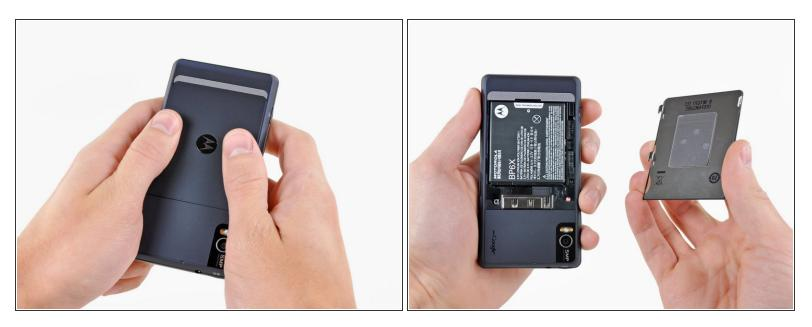
• The battery cover comes off without much fuss, and we're on our way to tearing this phone apart!
