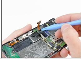
This Droid 2 opening tool gets a workout disconnecting the antenna, display data ribbon cable, and power/volume button ribbon cable from the motherboard.
