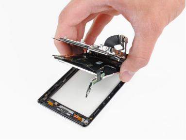
After disconnecting the digitizer ribbon cable and lifting out the earpiece, the front panel can be separated from the rest of the phone.
