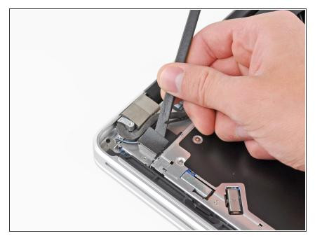
Use the flat end of a spudger to peel the thin plastic cover off the top and sides of the Bluetooth board housing.
