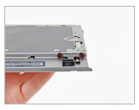
Remove the two 2.2 mm Phillips screws securing the Bluetooth board to the side of the optical drive.
