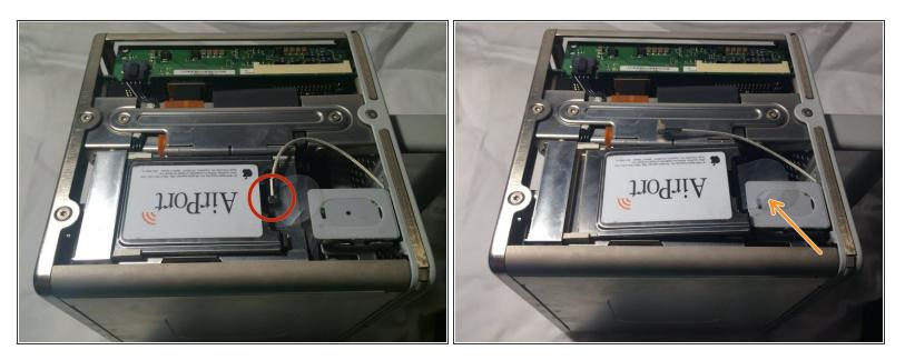
• Pull outwards on the antenna cable.
