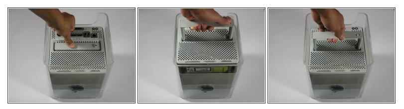
• Release the handle at the bottom of the Power Mac G4 Cube by pushing it down. Slowly pull out the cube by holding the end of the handle.
