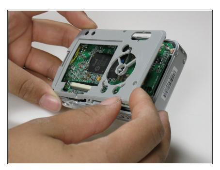
• Pull the inner casing off of the camera.
