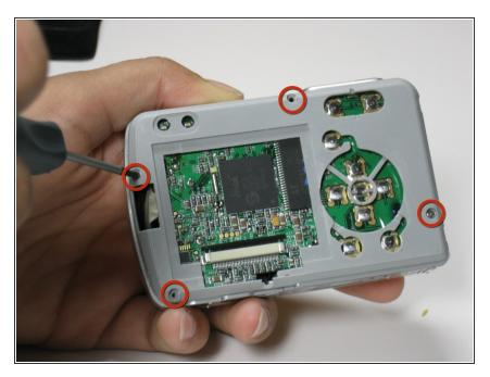
• Unscrew and remove the four (6 mm) screws on the inside casing.
