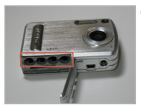
Remove the batteries from the camera.
