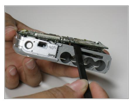
Use a spudger to pry up all four sides of the logic board and slide it out of the camera.
