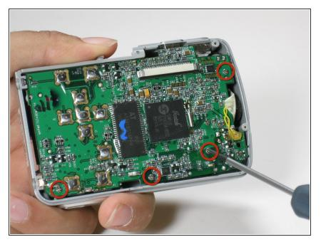
• Unscrew and remove the four (4mm) screws from the logic board.
