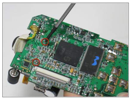
Unscrew and remove the two (5mm) screws from the logic board to the far left.
