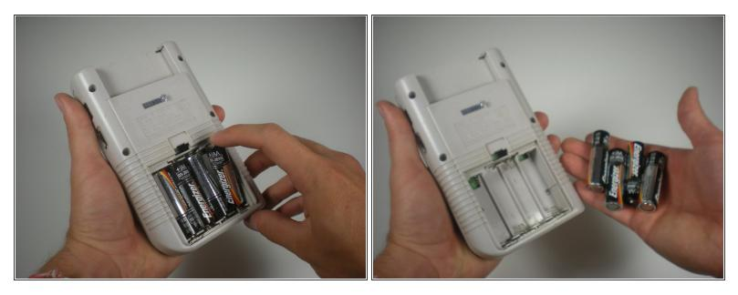
Use a fingernail to pry each battery outward from the positive (+) terminal to remove them.
