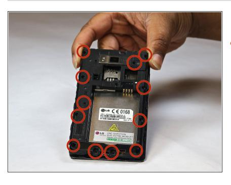
Remove the twelve screws using the Phillips 000 screwdriver.
