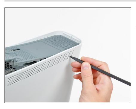
Use the tip of your spudger to release the clip on the top vent nearest the back of the Xbox's upper case.
