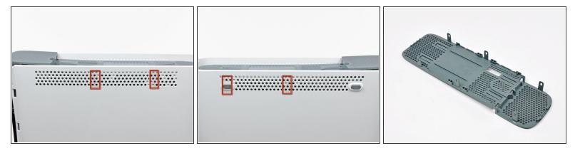
in the next few steps, you will use the tip of a spudger or the finger of an Xbox 360 opening tool to release the clips along the left and right sides of the top vent. Their locations are highlighted in red.
