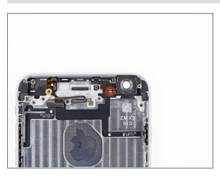
Remove the single 1.3 mm Phillips #00 screw securing the power button cable bracket to the rear case.
