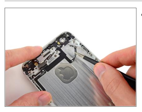
Pull the power button switch out of its recess on the rear case with a pair of tweezers.
