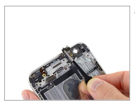
Carefully grasp the bracket with a pair of tweezers and remove it from the iPhone.
