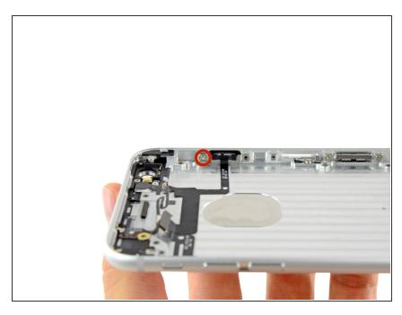
Remove the single 2.1 mm Phillips #00 screw securing the power button switch to the rear case.
