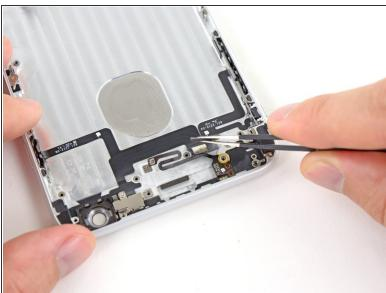
Use a pair of tweezers to peel the single adhesive tab that resides on top of both the power button and audio control/rocker switch cable connectors.
