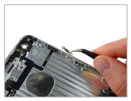
Grasp the metal bracket covering the power button switch with a pair of tweezers and remove it from the iPhone.
