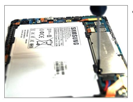
Remove the 6 screws securing battery.
