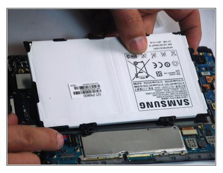
• Remove the original battery, replace it with a new one.
