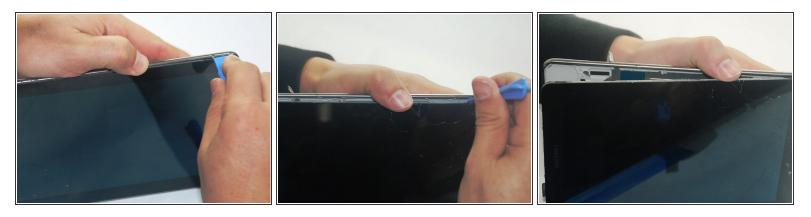
• Using the prying tool, pry the silver binding from around tablet from glass edge. You will need to go around the device several times applying some force before it comes off.
