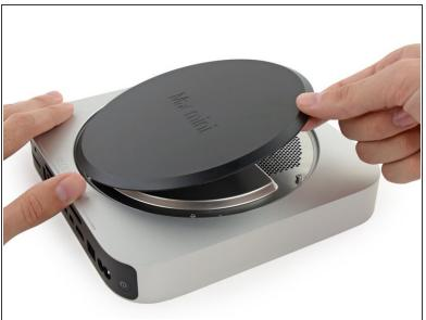
Lift and remove the bottom cover.
