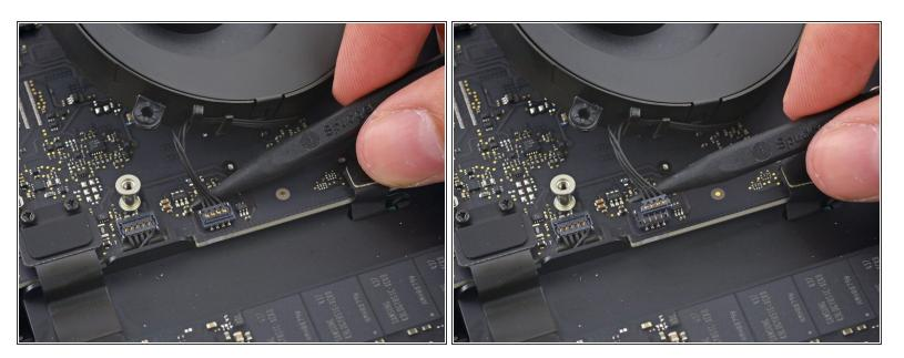
• Use the point of a spudger to lift the fan connector straight up out of its socket on the logic board.
