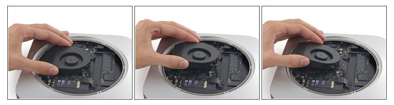
(i) The fan connector is trapped under the edge of the fan and cannot be disconnected until the fan is moved.
