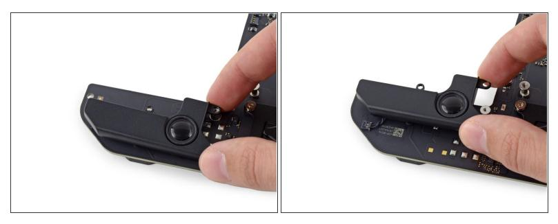
A Do not attempt to remove the speaker entirely as it is still attached to the logic board.
