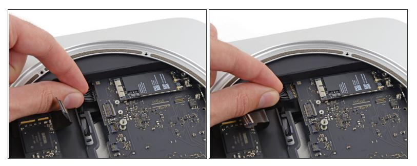
• Pull the DC-In cable connector straight out of its socket on the logic board.
