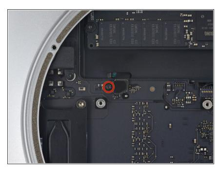
Remove the 2.6 mm T6 screw securing the SATA cable connector bracket.
