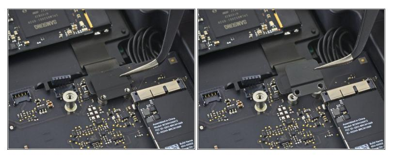
• Remove the PCIe SSD cable bracket.
