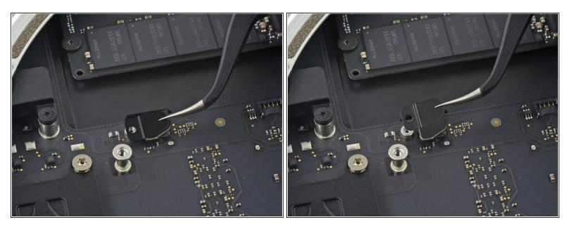
• Remove the SATA cable connector bracket.
