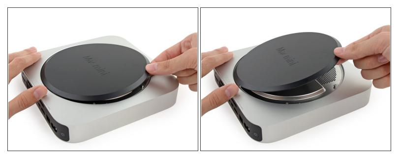
• Lift and remove the bottom cover.
