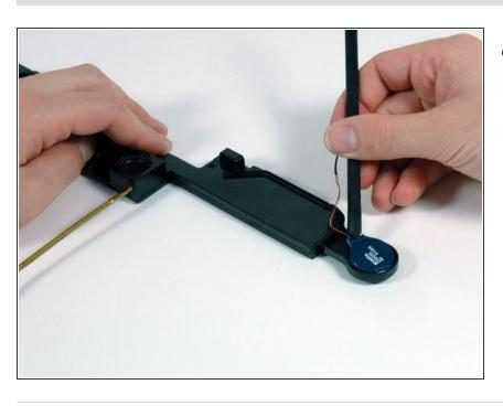
Use a spudger to pry up the PRAM battery from its housing on the left speaker assembly.
