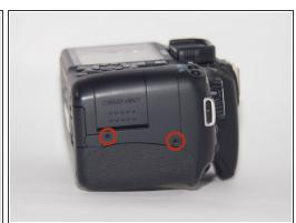
Use a 00 Phillips head screwdriver to unscrew these screws.
