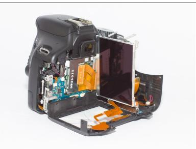
• Lift the broken screen and remove it. Then replace the new screen and attach the tabs that were removed in step 5. Replace the battery and turn on the camera to make sure it works.
