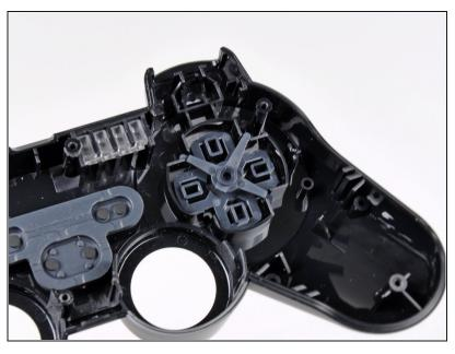
i The D-pad has a three-armed plastic piece that must be installed as shown before installing the rubber button pad for it to work properly.
