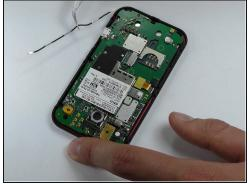
• Pry the antenna off using the metal spudger and <u>tweezers</u> and replace with the new one.
