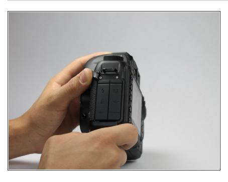
Peel back the rubber cover above the in/out ports to reveal two screw heads.
