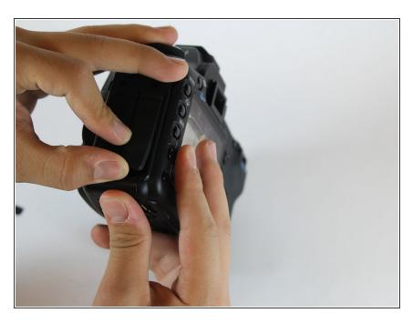
Lift the rubber flap covering the input/output jacks.
