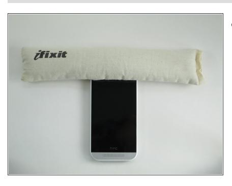
Heat up the top grey speaker plate with the iFixit iOpener for two minutes.
