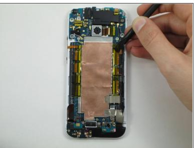
Peel off the long yellow pieces of tape on the right and left side of the copper plate.
