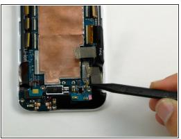
Use the pointed end of the spudger to pop off the four antenna connectors. Three are located on the top left corner of the motherboard and one on the bottom right.
