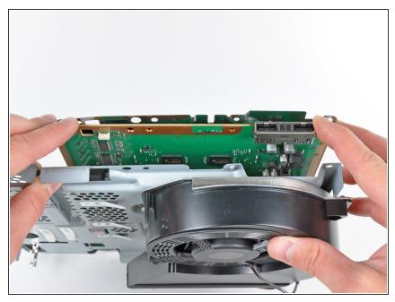
i If necessary, gently pry the motherboard off the top shield near the heat sink and its shroud.
