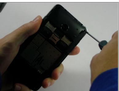
Use a screwdriver to remove each of the four screws.
