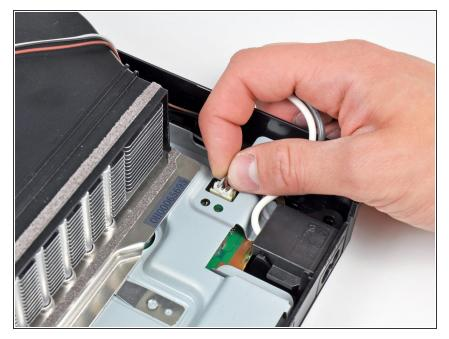
Pull the fan cables upward to lift the fan connector up and out of its socket on the motherboard.
