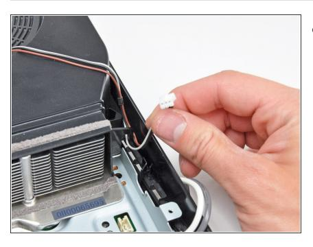
De-route the fan cables from under the plastic hook molded into the fan shroud.
