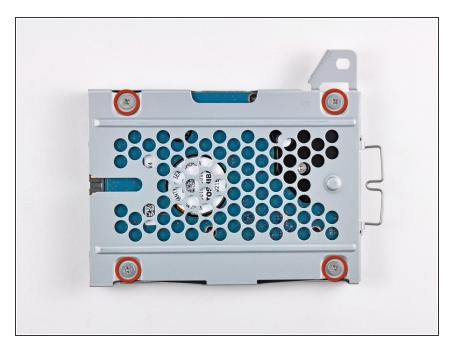
Remove the four 4.3 mm Phillips screws securing the hard drive to its tray.
