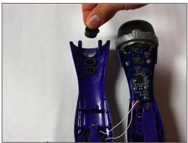
Remove the buttons by pushing them out from the front of the device. Clean or replace them as needed and place them back into the appropriate slots.
