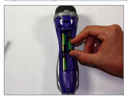
• Remove the 3 AAA batteries from the device.
