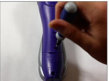
Remove the back panel of the device by unscrewing the single #8 11.6 mm Flathead screw on the back of the device.
