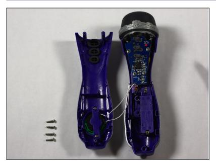
Keeping all wires connected to their attachments, place the front half of the device face down.
