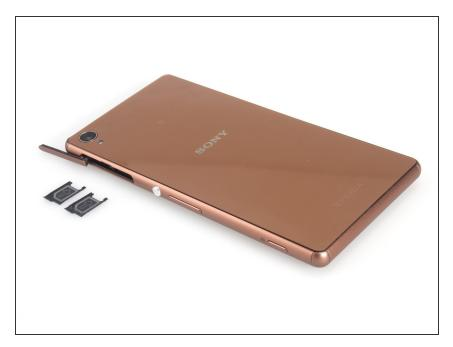
Power off the phone and remove two SIM card trays before headphone jack replacement.
