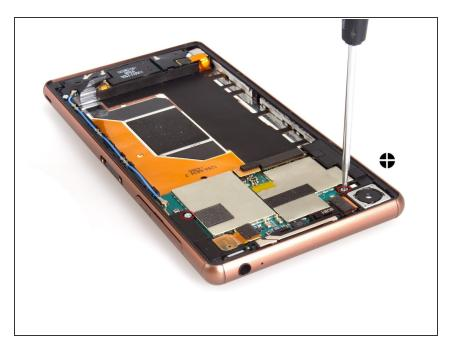
Twist off two screws by Philips screwdriver at first.
