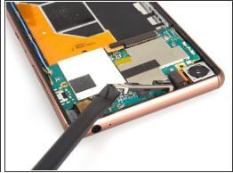
Remove three pieces of securing bracket.
