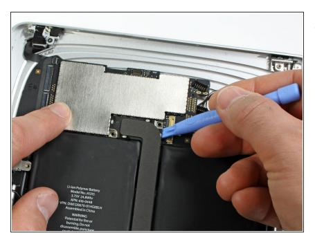
Use the edge of an iPod opening tool to carefully pry the dock cable connector straight up off the logic board.
