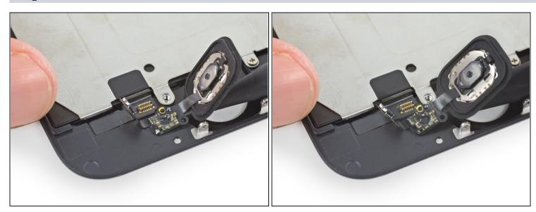
• Use the point of a spudger to carefully separate the home button cable from the adhesive securing it to the front panel.
