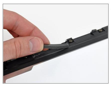
if present, remove the strip of foam tape along the long edge of the display assembly near the digitizer cable.
