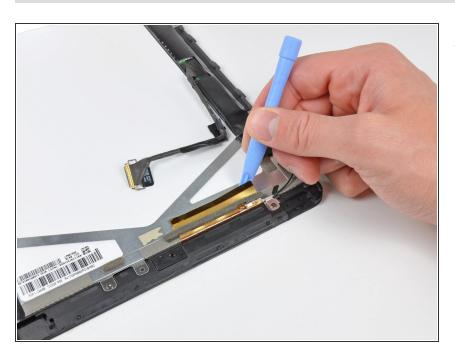
Use the edge of an iPod opening tool to peel the antenna off the adhesive securing it to the top edge of the display.
