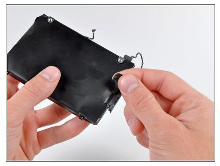
Remove the strip of tape connecting the hard drive cable to the hard drive.
