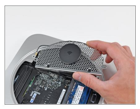
Remove the antenna plate from the mini.
