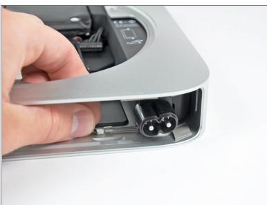
Pull the silver metal AC-In socket retainer away from the side of the outer case and remove it from the mini.
