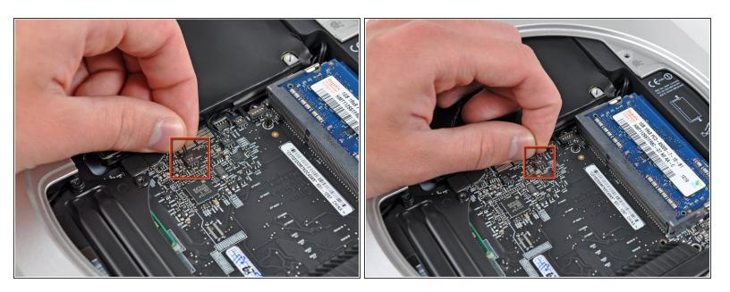
Carefully pull the wires for both hard drive thermal sensors upward to lift their connectors up and out of the sockets on the logic board.
