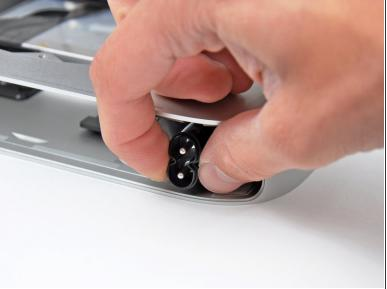
Rotate the AC-In connector 90 degrees counter-clockwise.
