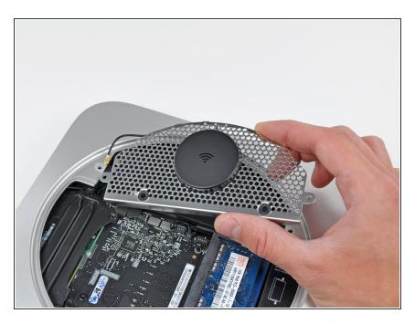
Remove the antenna plate from the mini.
