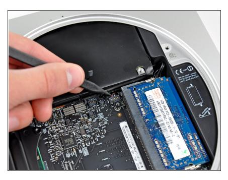
Use the tip of a spudger to lift the IR sensor connector up and out of its socket on the logic board.
