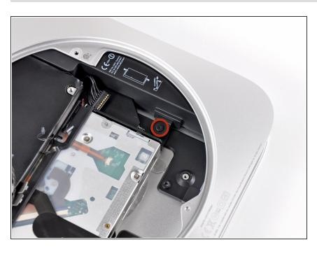
Remove the 7.9 mm T6 Torx screw securing the power supply and optical drive to the outer case.
