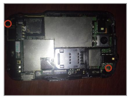
remove 2 phillips screws and remove motherboard
